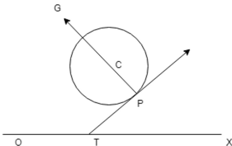
If a length  $PC$  equal to  $\rho$  is measured from  $P$  along the positive direction of the normal, the point  $C$  is called the *centre of curvature* at  $P$ , and the circle with centre  $C$  and radius  $CP$  is called the *circle of curvature* at  $P$ .
